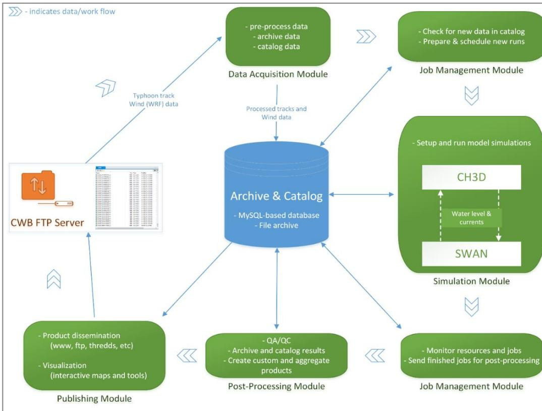
**Figure 2. All modules of the CH3D-SWAN forecasting system.**
