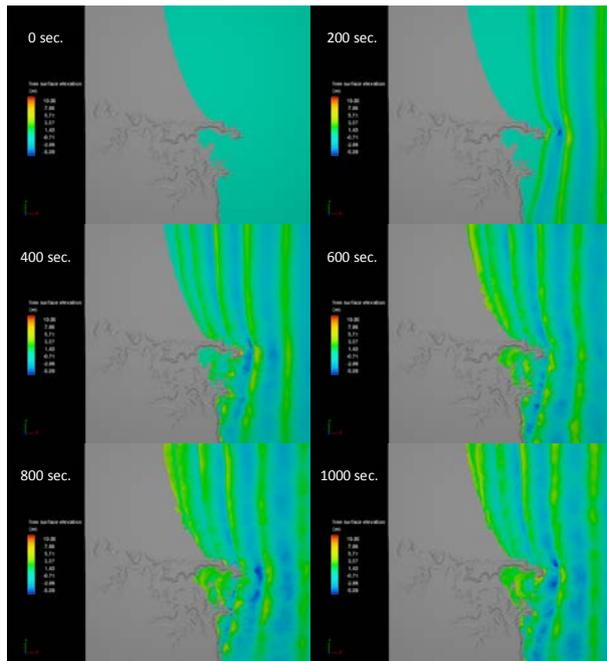
**Fig. 1.** The simulation result of water level changes around Su-ao harbor area.
